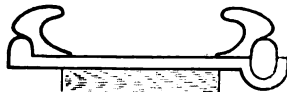
Cross Section, Michelin Quick Detachable Rim, with rings adaptable to clincher type tire
